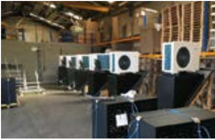
In our workshop heat pumps are being connected.
